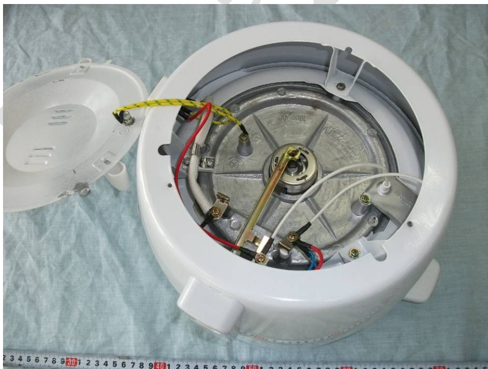
Figure A-5 Electrical Circuit Photo (RC-16A)
