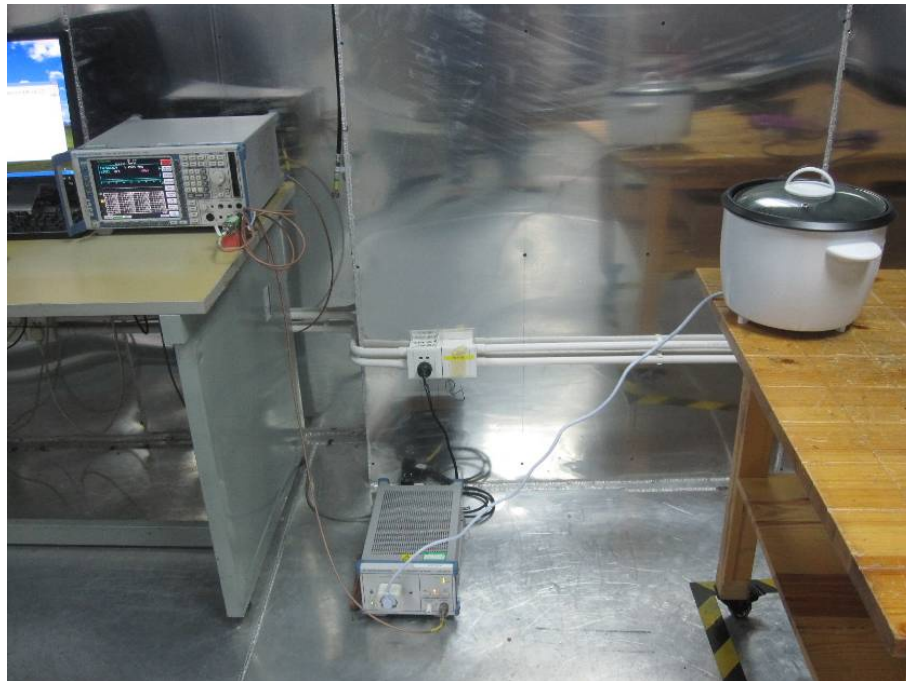
Figure B-1 Setup for conducted emission
