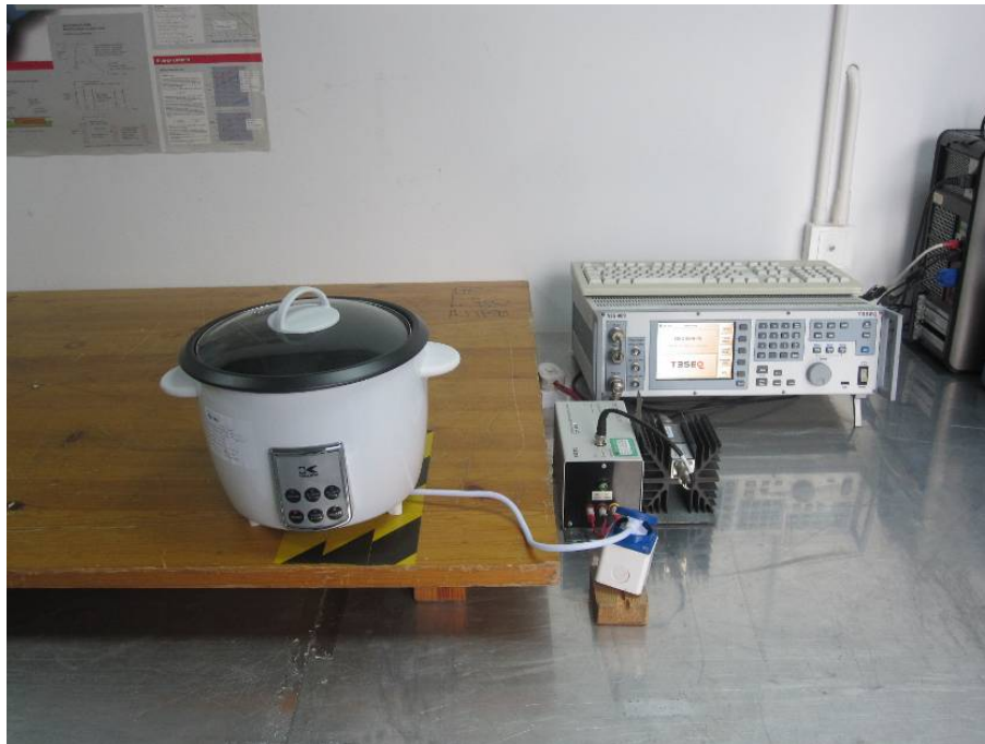
Figure B-7 Setup for Conducted Immunity
