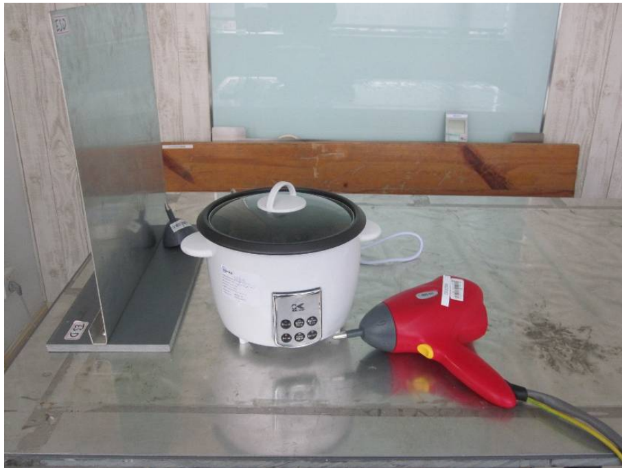
Figure B-5 Setup for ESD
