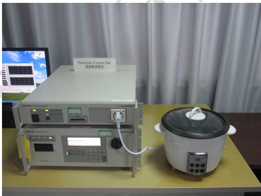
Figure B-3 Setup for disturbance power
