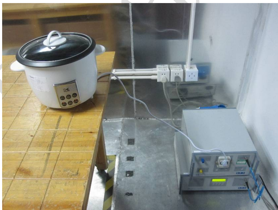
Figure B-1 Setup for conducted emission
